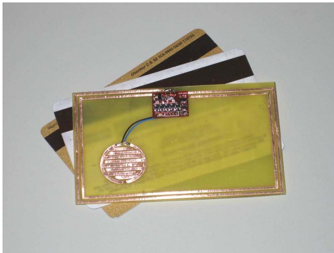
Figure 5 Touch enhanced UHF near-field RFID tag in the form factor of a credit card.
